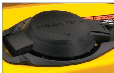
Quick latch fuel filler design
