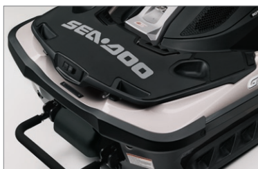
Reboarding platform with storage
